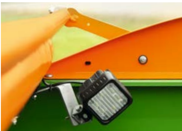
Lighting for the inside of the hopper
