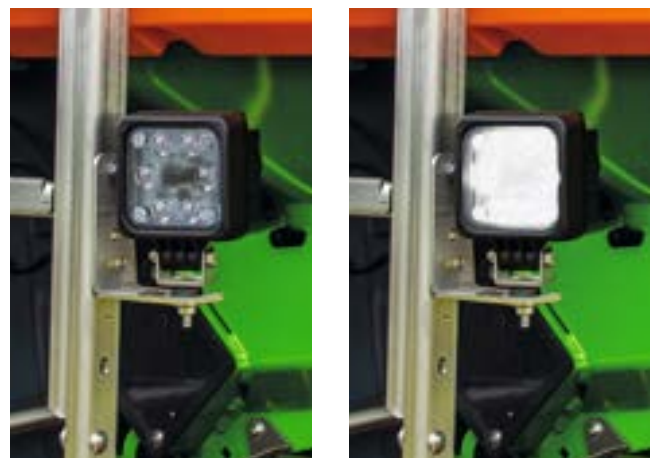
The pre-set capacity is achieved when the work lights comes on continuously.
