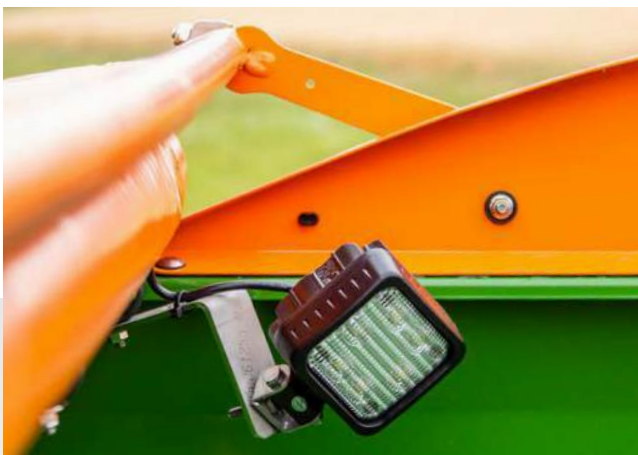
Lighting for the inside of the hopper
