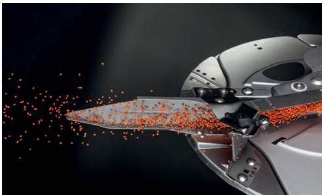
AutoTS – setting for normal spreading
