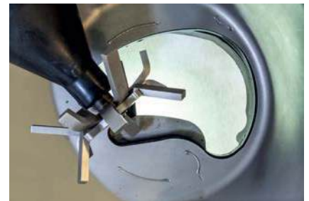
Stage 3: hopper aperture wide open
