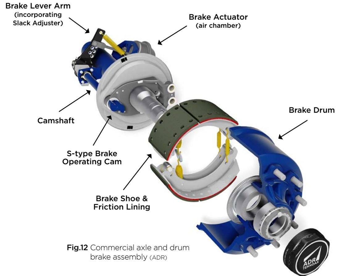
Fig.12 Commercial axle and drum brake assembly (ADR)
