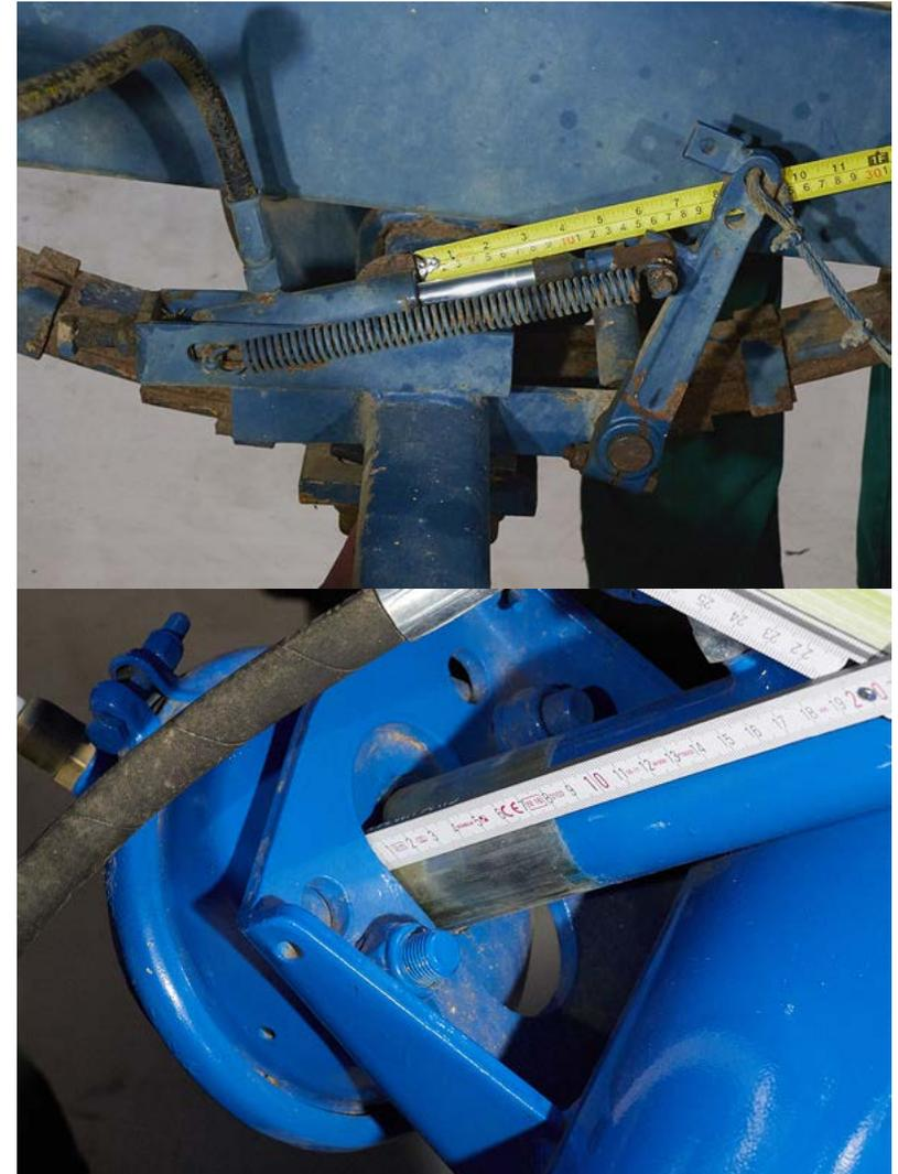
Fig.17 Excessive brake actuator free travel = No Brakes!
