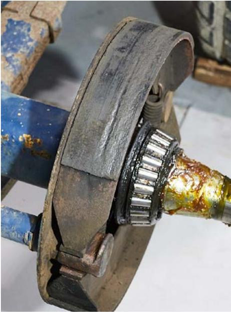
**Fig.29** Damaged/overheated trailer brake friction lining
