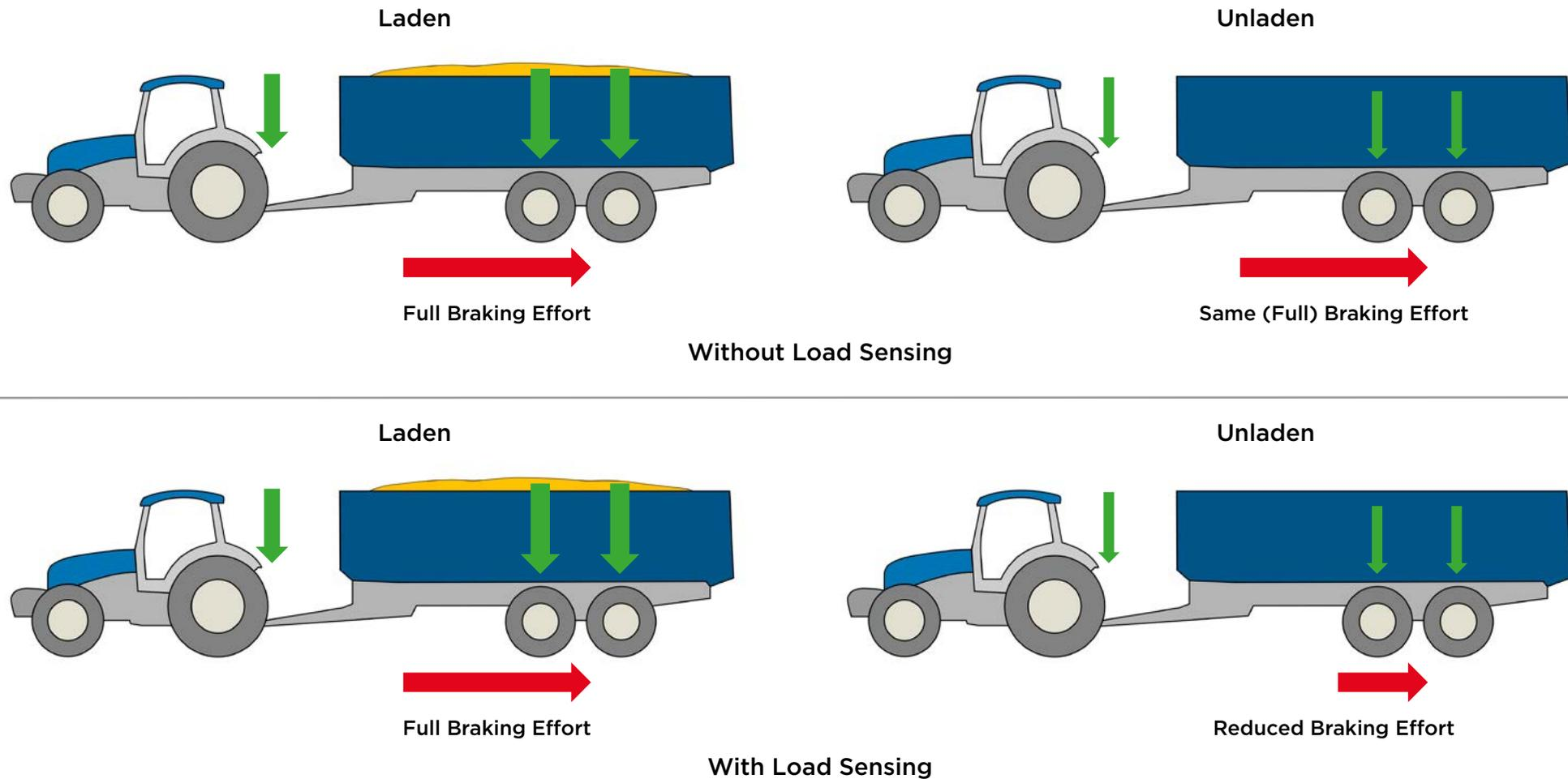
Fig.22 Trailer braking with and without Load Sensing
