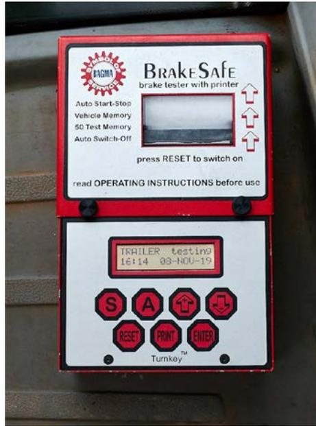
**Fig.30** BAGMA BrakeSafe braking performance tester
