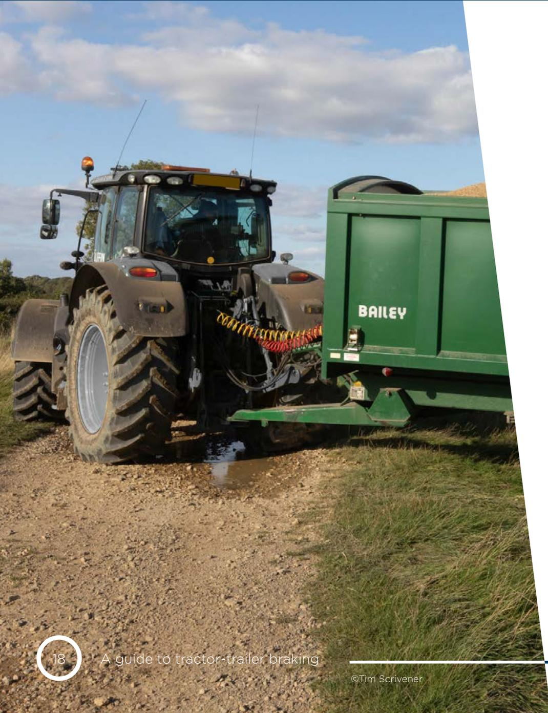
Pneumatic (air) braking systems are now much more popular and are probably the most common braking system used on larger tractor-trailer combinations. UK take-up has been helped by widespread fitment of trailer air brake equipment on newer, larger tractors
