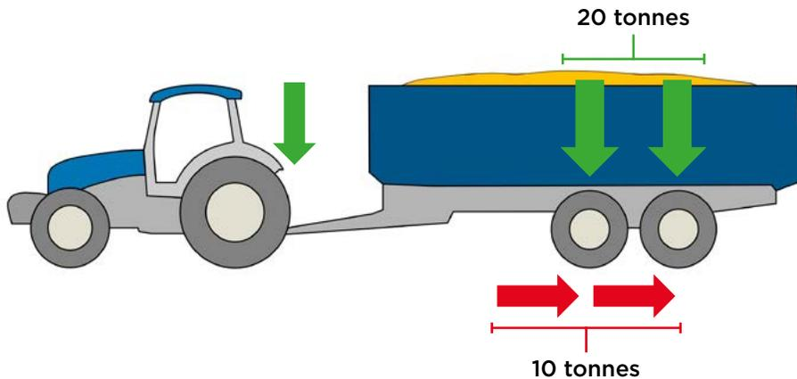
**Important:** Different vehicles may be lighter or heavier, but if each one can develop the same **Braking Efficiency**, they will each slow down and stop at the same rate. This is why road vehicle regulations use braking efficiency to specify braking system performance levels.
