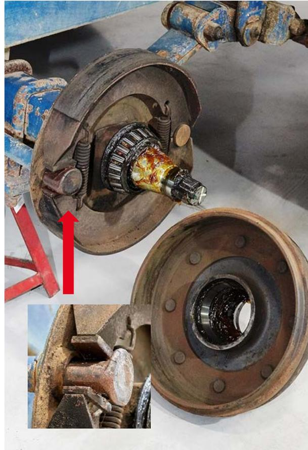
**Fig.13** Example Ag. Spec brake and drum - Note 'Flat'-type operating cam (arrowed & inset)
